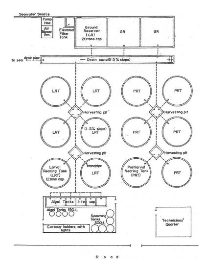
Fig. 11. A sample layout of a prawn hatchery.
