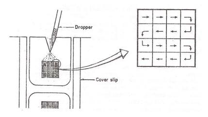
Fig. 19. Loading algal sample into the hemacytometer. The enlarged portion at the right shows the direction (arrows) for counting algae in areas AB, C or D under the microscope.
