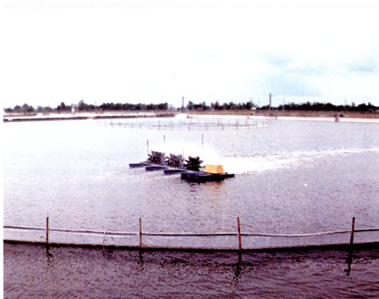
Fig. 6. The long-arm paddle wheel provides aeration and circulation
