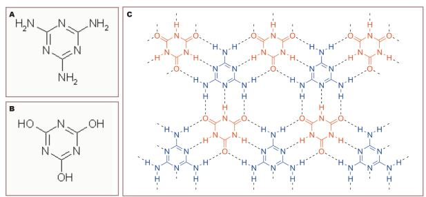
Figure 5.1. Chemical structures of (A) Melanine, (B) Cyanuric Acid and (C) Melamine Cyanurate Crystals
